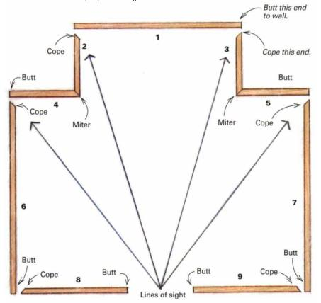
**Coped joints.** The first piece is butted to the wall. The second piece is mitered as for an inside corner, but the mitered end is cut off where it meets the molding face, leaving a negative of the profile that fits perfectly over the butted piece.
